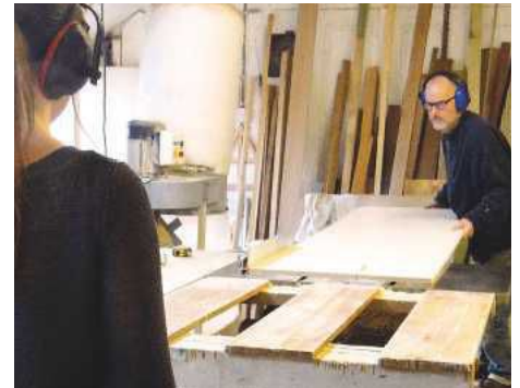
▲ Pic.3 You'll notice that Richard works with saw guards removed and you might reach for a pen. It worried me too in the beginning: I'm used to it now. Richard is fully familiar with working this way and is well aware of personal safety. Like this he can see clearly what the blade is doing. Perhaps he is more in control. But for anyone less experienced than Richard, this might be hazardous and is not to be tried at home. Good dust extraction keeps the air clear
